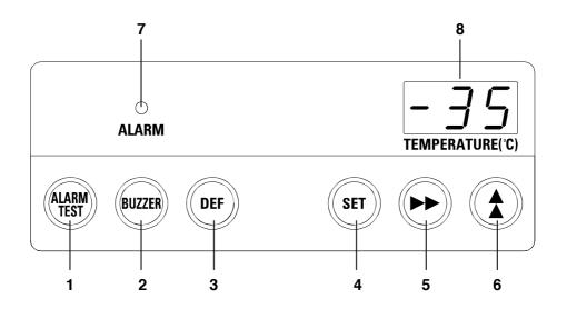
**1. Alarm test key (ALARM TEST):** Test key for alarm device. By pressing this key, the alarm lamp is flashed, remote alarm is activated and buzzer sound. This means all alarm function operate correctly.
